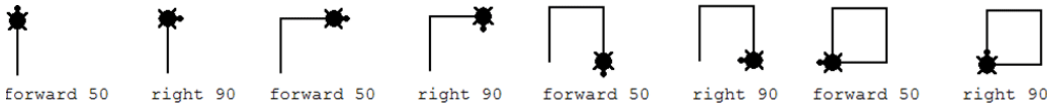
Figure 1. An example of a Logo program, drawing a square (with ‘pen down’ already called).
